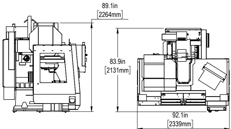
\*All Height Dimensions Based on Suggested Leveling Pad Height
