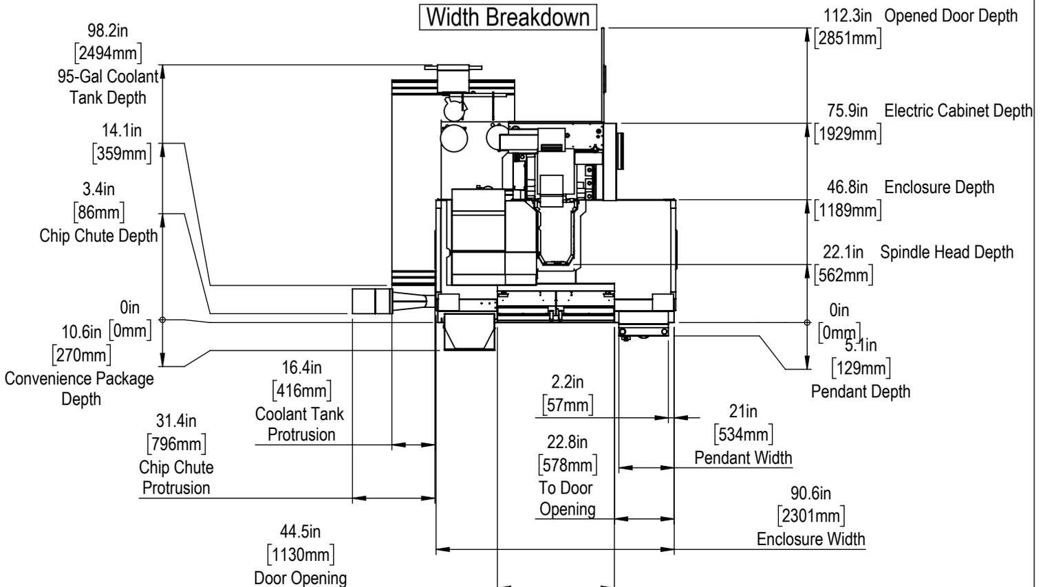
Maintain 3 feet [915mm] clearance to the nearest obstruction around all sides of machine perimeter for maintenance access
