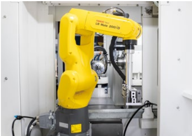
FANUC LR Mate 200iD Robot Loader (TG-5)
