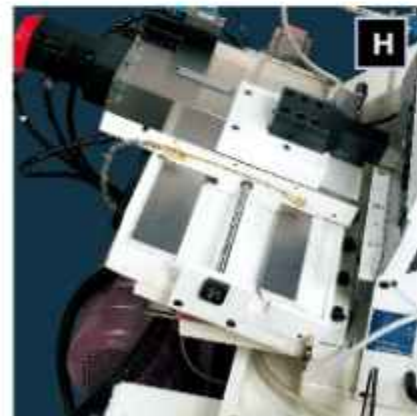
Stable Grinding Wheel Auto-Dressing Unit (For I Axis above) The lower slideways of the grinding wheel dressing unit is of a concave dovetail structure. This combines with extra large slideways for greatly upgrading the stability of the grinding wheel unit.
