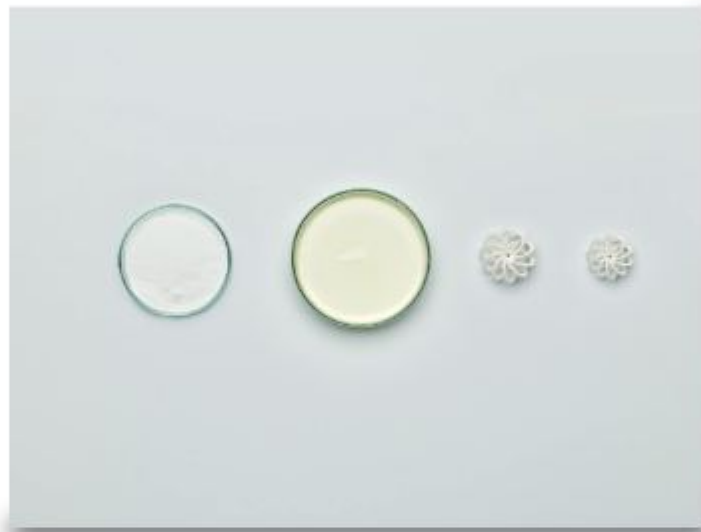
From powder to ceramic 3D printed and sintered part
