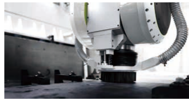
NC controllable telescopic suction hood around spindle
