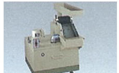
COOLANT SYSTEM WITH MAGNETIC SEPARATOR
