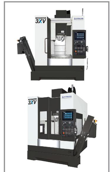
**Quality Components Throughout** - THK heavy duty cross linear guides, fine pitch ballscrews, high grade servo motors, feedback encoder and Kitamura's high precision assembly technology allows for the highest accuracy and smoothest possible motion on X, Y & Z axes. ±1µm repeatability is achievable.
