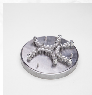
3 abutments in CoCr built in 3.20 h Post processing: connectors milling
